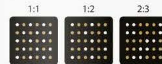
Examples of custom lasing ratios ● -1570 laser ● - CO 2 laser
